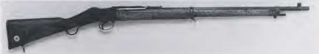
Figure 27 The Martini-Enfield rifle Mark II, W.A. Pattern. One of the 1150 Mark I and II rifles shipped here from the Tower between 1898 – 1901. The rifle still has its spring steel foresight protector in place. (Photo D. Elford).
